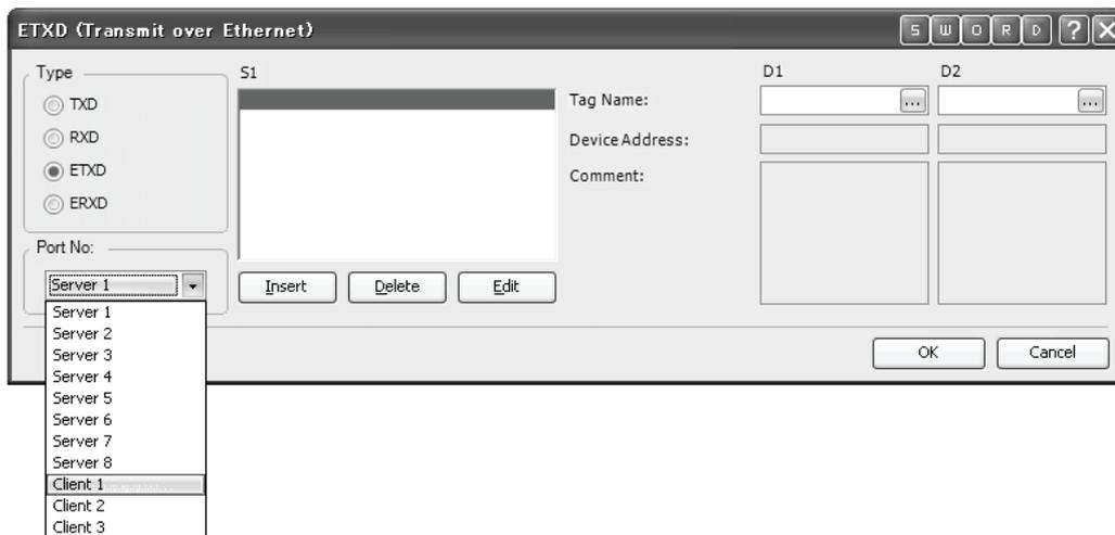
Select ETXD (Transmit over Ethernet) to transmit data or ERXD (Receive over Ethernet) to receive data as the instruction type. Select the client connection from 1 through 3 and designate S1, D1, and D2. Click **OK** button to close the dialog box.
