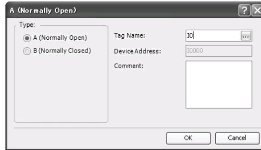
A NO contact of input I0 is programmed in the first column of the first ladder line.
