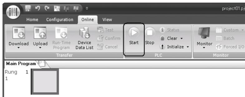
4. Click the **Start** button to start operation, then the start control special internal relay M8000 is turned on.
