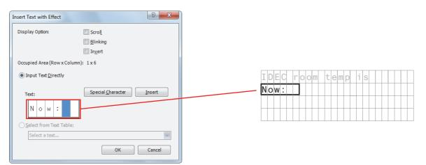
**8.** After the settings are configured, click **OK**. The configured content is displayed on the LCD screen area.
