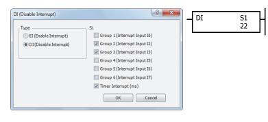
The total of selected interrupt inputs and timer interrupt is shown as source device S1.
