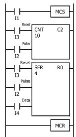
When input I1 is on, the MCS is not executed so that the counter and shift register are executed according to the actual status of subsequent inputs I2 through I4.
