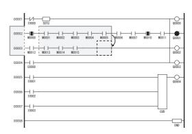
The cursor moves to the start of the next rung. The ladder program display screen changes as shown below.
