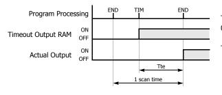
Timeout output error is equal to Tte (behind error) and can be between 0 and one scan time.
