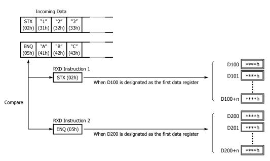
The incoming data is divided, converted, and stored to data registers according to the receive format. Start delimiters are not stored to data registers.
