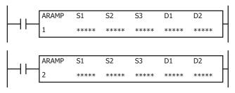
The ARAMP instructions output pulses with the frequency change function according to the information in the frequency table.
