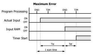
When the input turns on immediately after END processing, Tie is almost equal to one scan time. Then the timer input error is Tie + Tet = one scan time + Tet (behind error) and is at its maximum.
