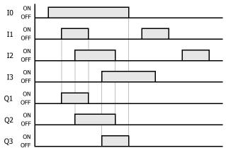
When both inputs I0 and I1 are on, output Q1 is turned on.
