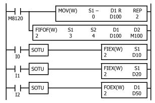
M8120 is the initialize pulse special internal relay.
