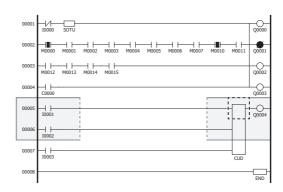
**2.** With the cursor at the position of the CUD instruction, press the *integral* (OK) button. The details screen is displayed.
