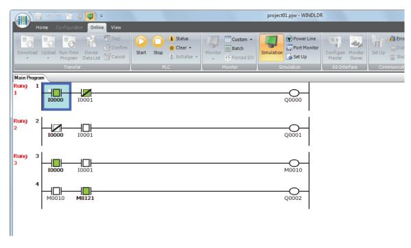
To change an input status, place the mouse pointer on the input and right-click the mouse. In the pop-up menu, select Set or Reset to set or reset the input.
