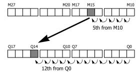
As a result, when input I0 is on, the ON/OFF status of internal relay M15 is moved to output Q14.
