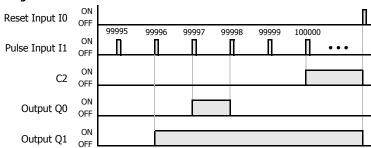
Output Q0 is on when counter C2 current value is 99997.
