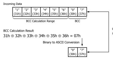
Comparison result is true to indicate that data is received correctly.
