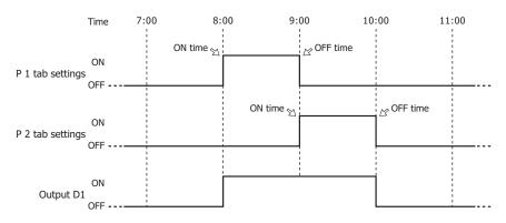
If **ON time** is 9:00 and **OFF time** is 10:00 on the **P 1** tab and **ON time** is 8:00 and **OFF time** is 9:00 on the **P 2** tab, the 9:00 setting is duplicated on the two tabs and **ON time** for the **P 1** tab is disabled. In this situation, the output is on from 8:00 to 9:00.
