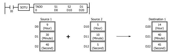
When the result exceeds 23:59:59, the resultant hour data is subtracted by 24, turning on special internal relay M8003 (carry).
