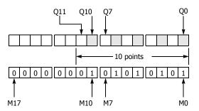
This program will invert the status of the shaded outputs on the left from on to off, and those not shaded from off to on.
