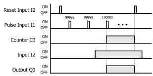
• The preset value 0 through 4,294,967,295 can be designated using a data register D0 through D1998; then the data of the data registers becomes the preset value.
