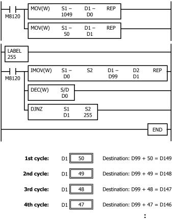
M8120 is the initialize pulse special internal relay. At start-up, MOV instructions store initial data.  $1049 \rightarrow D0$  to store the value for the first cycle.  $50 \rightarrow D1$  to determine the jump cycles.
