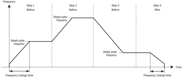
When the initialization input specified by S2 is turned on, the initial values configured in the WindLDR ARAMP instruction are stored in the control registers.
