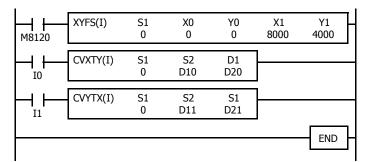
M8120 is the initialize pulse special internal relay.
