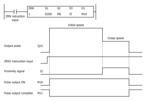
When the ZRN1 instruction changes from off to on, pulses are output at the initial pulse frequency. When pulse output starts, M10 turns on and M11 turns off. When I2 changes from off to on, pulses are output at the creep pulse frequency. When I2 changes from on to off, pulse output stops. When pulse output stops, M10 turns off and M11 turns on.
