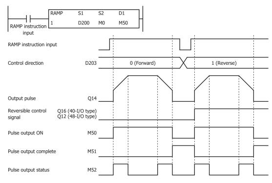
[RAMP1 instruction, S1 is specified as D200, D1 is specified as internal relay M50]
