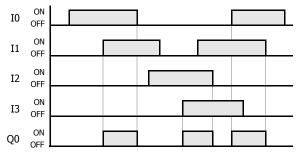
When both inputs I0 and I1 are on or both inputs I2 and I3 are on, output Q0 is on.
