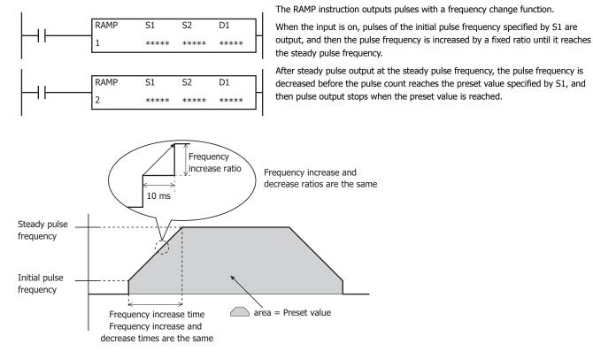
**Note:** Configure multiple PULS (pulse output), PWM (pulse width modulation), RAMP (trapezoidal control), and ARAMP (RAMP with table) instructions so that they do not share the same pulse output port.
