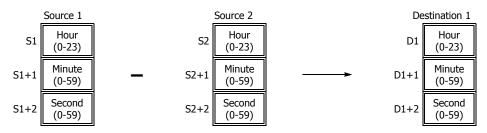
Hour data can be 0 through 23. Minute and second data can be 0 through 59.
