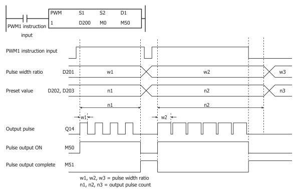
When the PWM1 instruction input changes from off to on, M50 turns on and pulses with the width ratio configured by D201 are output. When the number of pulses configured by D202 and D203 are output, pulse output stops. If the value of D201 changes during pulse output, pulses are output with the width ratio based on that value.
