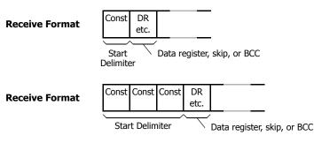
Note: Constants following data register, skip, or BCC are not considered start delimiter even if these are in the first five bytes of the receive format.
