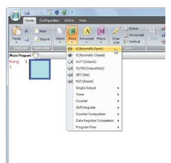
2. Move the mouse pointer to the first column of the first line where you want to insert a NO contact, and click the left mouse button.
