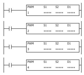
The PWM instructions output pulses at the specified frequency and duty cycle from the output port.
