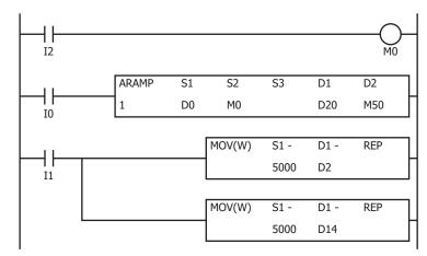
When I2 turns on, the initialization input (M0) is turned on and the ARAMP instruction control register values are initialized
