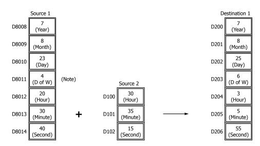
When the result exceeds 23:59:59, the resultant hour data is subtracted by a multiple of 24 and the day data is incremented.
