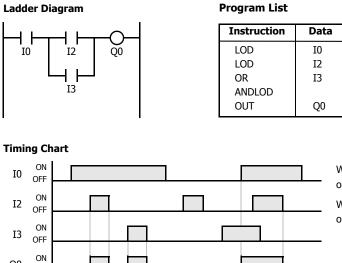
When input I0 is on and either input I2 or I3 is on, output Q0 is on.
