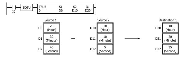
When the result is less than 00:00:00, 24 is added to the result, turning on special internal relay M8003 (borrow).
