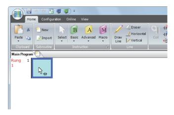
**Note:** Another method to insert a NO (or NC) contact is to move the mouse pointer where you want to insert the contact, and type A (or B). The Normally Open dialog box appears.
