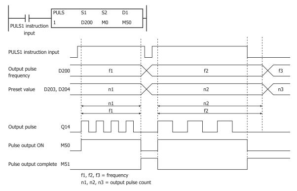
When the PULS1 instruction input changes from off to on, M50 turns on and pulses with the frequency configured by D200 are output. When the number of pulses configured by D202 and D203 are output, pulse output stops. If the value of D200 changes during pulse output, pulses are output with the frequency based on that value.
