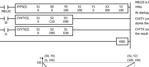
M8120 is the initialize pulse special internal relay.
