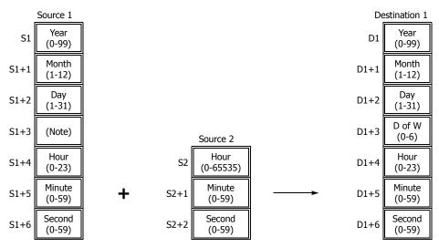
Note: Device S1+3 in source 1 is not used for execution and need not be designated.
