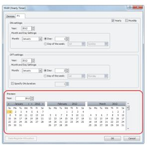
The preview shows the ON/OFF state for the output based on the settings configured on the parameter tabs in a calendar. The dates that are set to ON are highlighted in orange. Three months are shown at one time.
