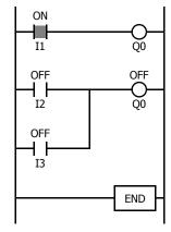
Programming multiple outputs of the same output number is not recommended. However, if doing so, it is good practice to separate the outputs with the JMP/JEND set of instructions, or the MCS/MCR set of instructions. These instructions are detailed later in this chapter.
