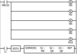
Ten outputs Q0 through Q11 are assigned to 10 internal relays M0 through M11.
