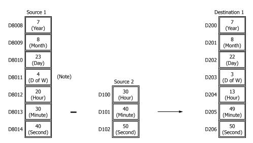
**Note:** D8011 in source 1 is not used for execution and does not need to be designated. The day of week is calculated automatically from the resultant year, month, and day, and stored to D203 of destination 1.
