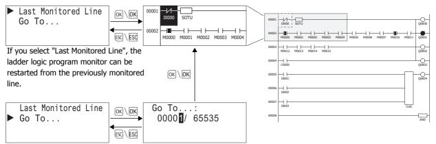
If you select "Go To..." and specify a ladder logic program monitor line, the ladder logic program is displayed with the specified line at the beginning.
