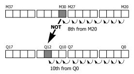
As a result, when input I0 is on, the ON/OFF status of internal relay M30 is inverted and moved to output Q12.
