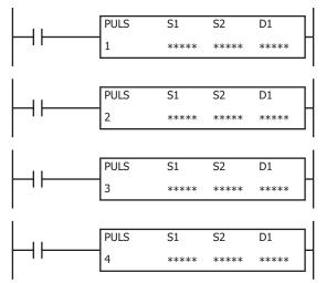
The PULS instructions output pulses of a specified frequency from the specified pulse output ports.
