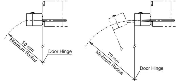
**Actuator Angle Adjustment for the HS9Z-A55**
