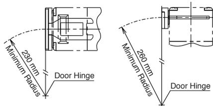
**When using the HS9Z-A55 Angle Adjustable Actuator**
