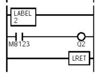
M8123 is the 10-msec clock special internal relay.
